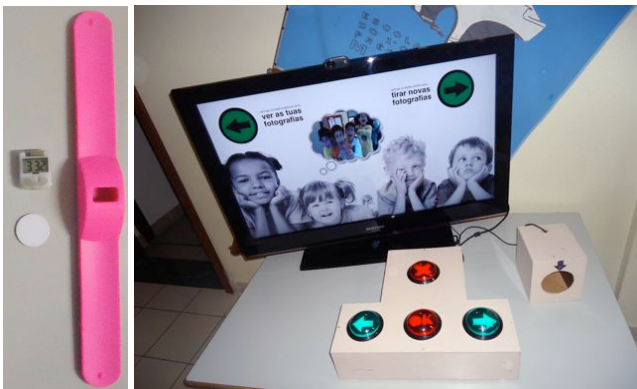
Figure 1. (left) Watch with RFID tag, (right) Playful Booth installation with navigation buttons and the RFID reader box
